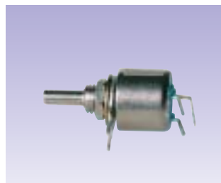
RV12YP5 全抵抗値: 100 ~ 2M / 定格電力: 0.5W at 40 / 電気的回転角: 270° / 使用温度範囲: - 10 ~ 85 Standard resistance range: 100 to 2M / Power rating: 0.5W at 40 / Adjustment travel: 270° / Temp. range: - 10 to 85
