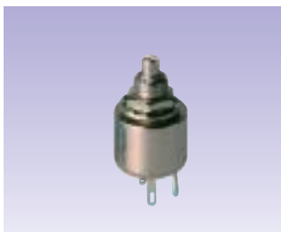
RV12YN 全抵抗値: 100 ~ 2M / 定格電力: 0.5W at 40 / 電気的回転角: 270° / 使用温度範囲: - 10 ~ 85 Standard resistance range: 100 to 2M / Power rating: 0.5W at 40 / Adjustment travel: 270° / Temp. range: - 10 to 85
