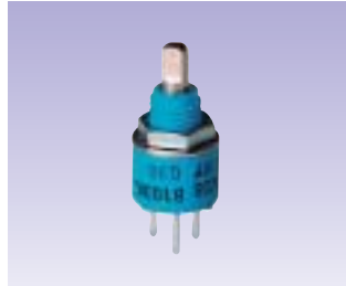
RV102YP 全抵抗値: 100 ~ 2M / 定格電力: 0.25W at 40 / 電気的回転角: 270° / 使用温度範囲: - 10 ~ 85 Standard resistance range: 100 to 2M / Power rating: 0.25W at 40 / Adjustment travel: 270° / Temp. range: - 10 to 85
